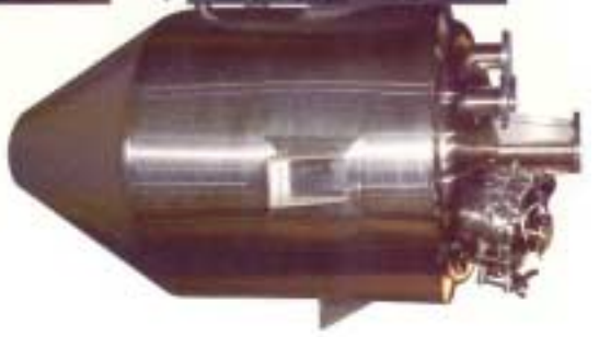
Hastelloy™ pharmaceutical reactor with A.S.M.E. half-pipe heat transfer surface on bottom cone.
